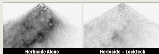
FIGURE 5 - EFFECT OF LOCKTECH ON DROPLETS. INCREASED “FOG” INDICATES MORE FINE DROPLETS. LOCKTECH TREATMENT SHOWS FEWER FINE DROPLETS.
