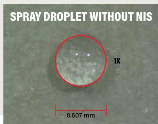
FIGURE 7 - DROPLET SPREAD OF WATER COMPARED TO SURFACTANT.
