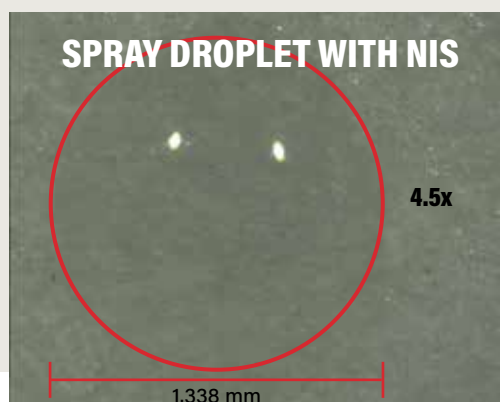
FIGURE 7 - DROPLET SPREAD OF WATER COMPARED TO SURFACTANT.
